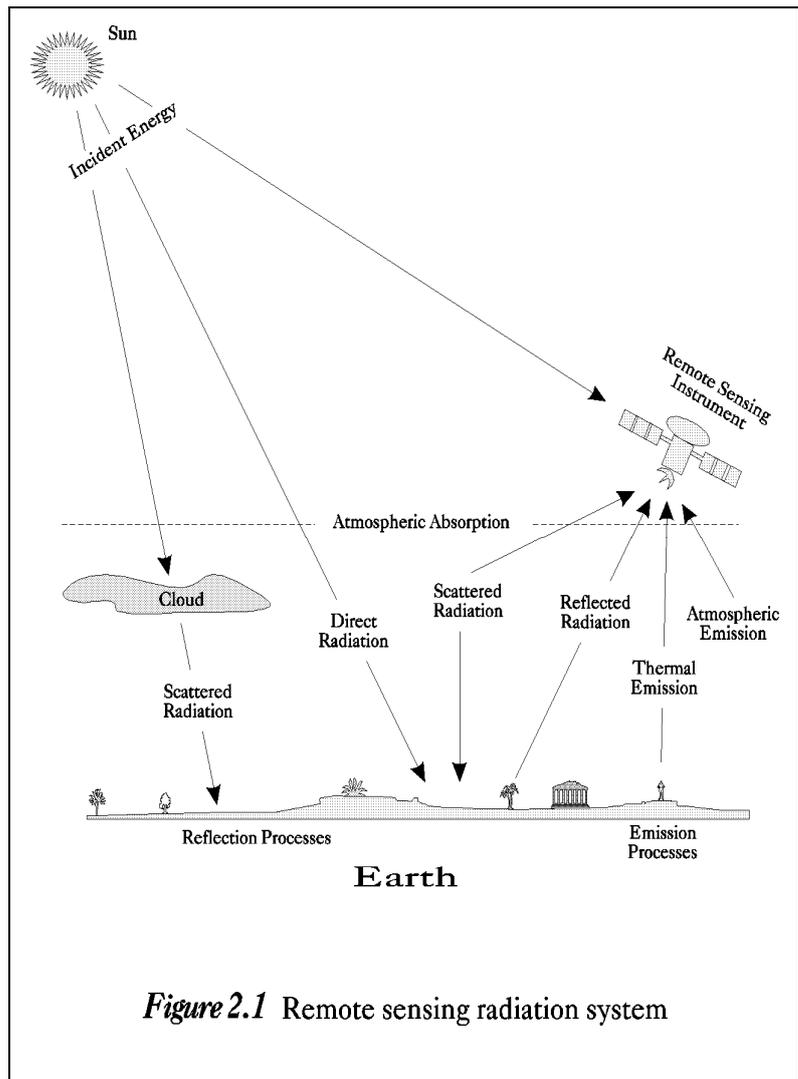
*Figure 2.1* Remote sensing radiation system
